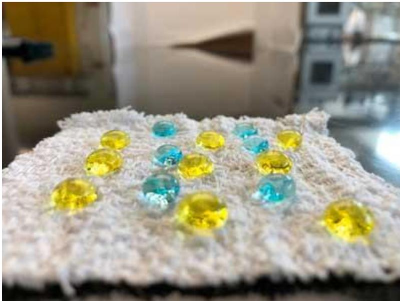
*The nanocoating on this fabric, when installed in air filtration systems, is capable of capturing airborne virus particles, trapping them on the filter's coating with zero reduction in air flow.*
